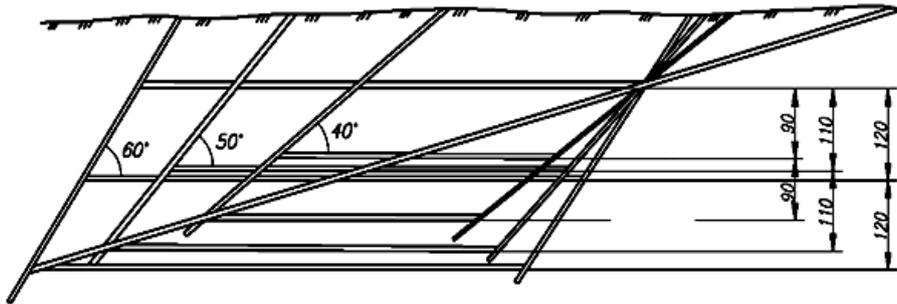
Figure 3 - Location of inclined shafts depending on the dip angle of the layers [3]
